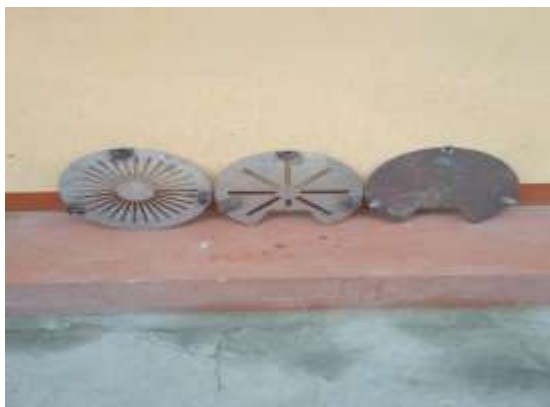
Figure 3. Types of discs that are fastened to the cutting blade (the first for corn grains, the second for foliar or dry hay).
